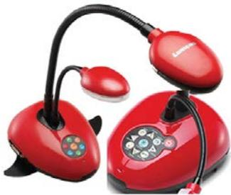
We have two brands of document cameras in our district. Lumens brand cameras will show your document when the projector is on without using software. You will switch between display of your document and display of your computer screen by pushing the source/enter button on the camera, or the source button on your projector.
